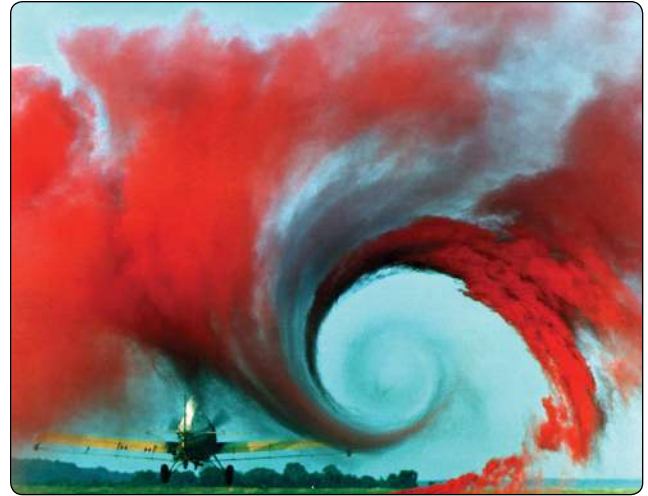
Figure 5-9. Wingtip vortex from a crop duster.
