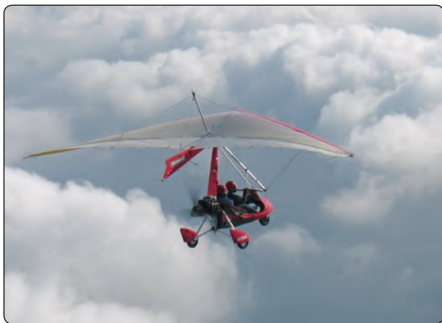
Figure 5-19. A weight-shift control aircraft.
