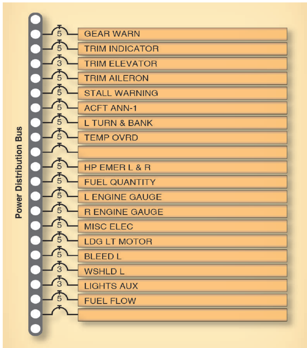
Figure 15-9. Typical individual power distribution bus.
