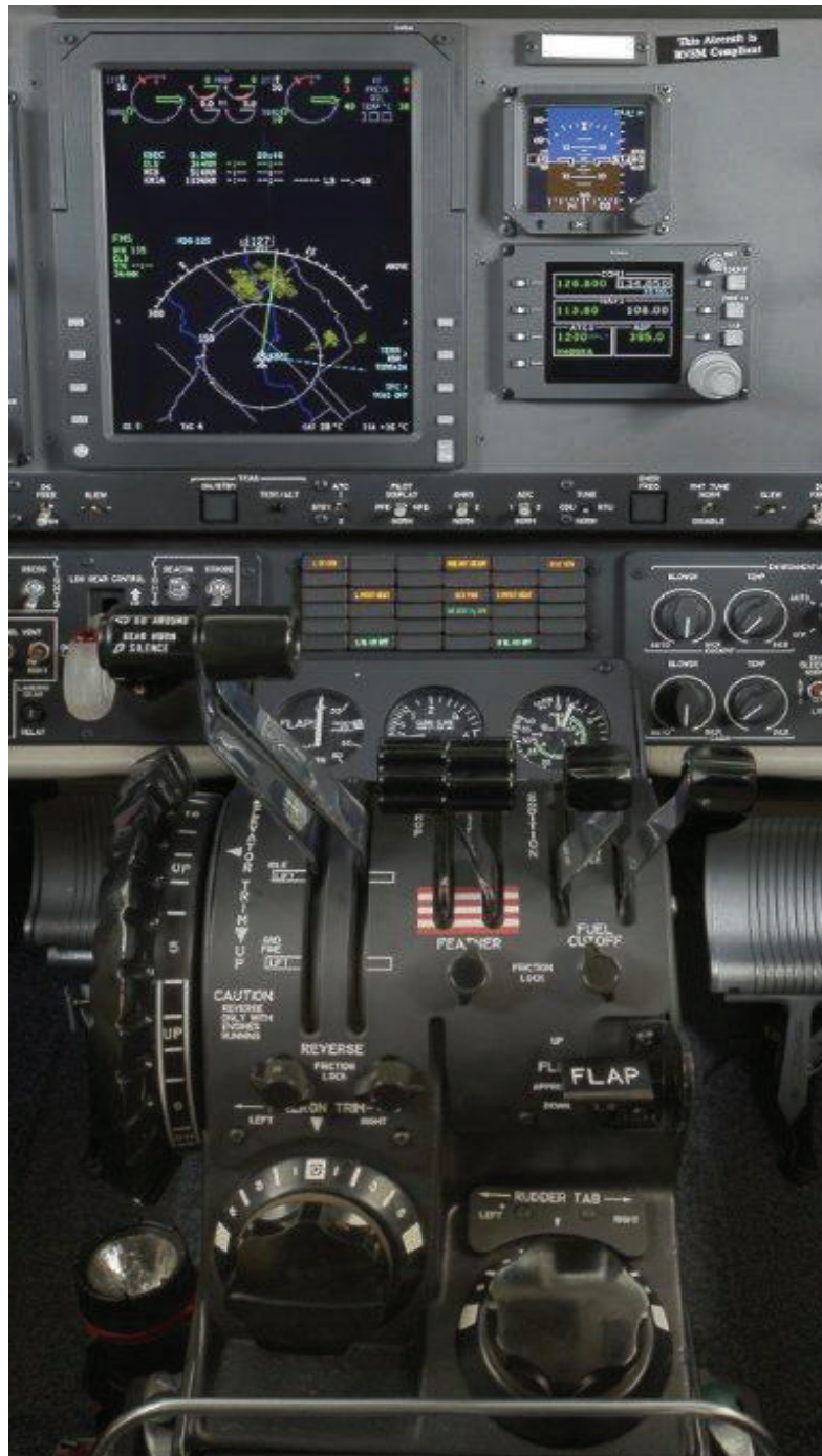
Figure 15-6. Powerplant controls—split-shaft/free turbine engine.
