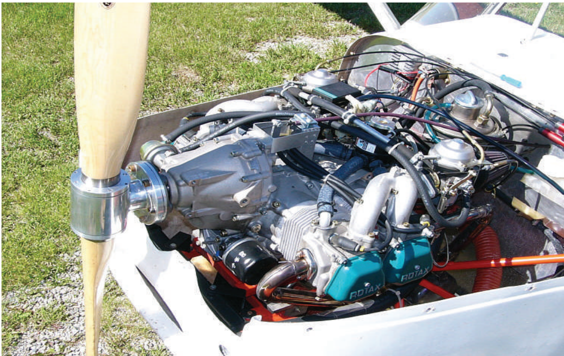
Figure 17-4. A water-cooled 4-cycle engine.
