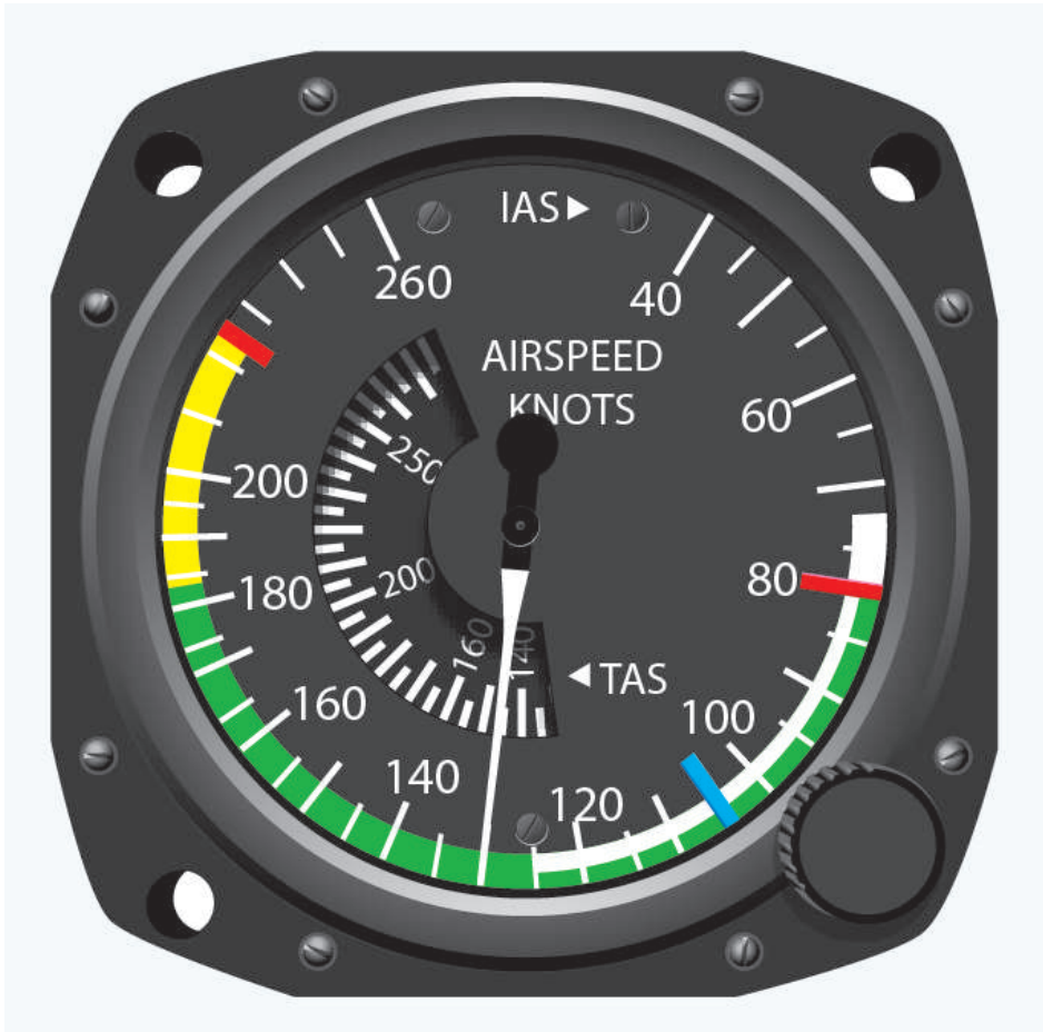
Figure 13-1. Airspeed indicator markings for a multiengine airplane
