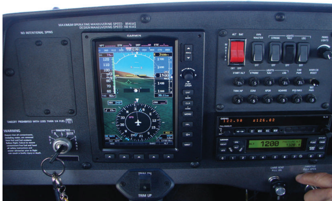
Figure 17-15. EFIS indication of level cruise flight.
