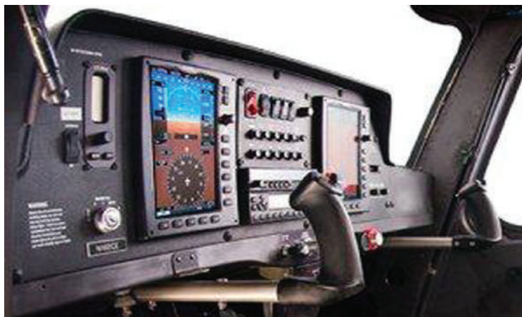
Figure 17-11. Stoke flight control with conventional engine controls.
