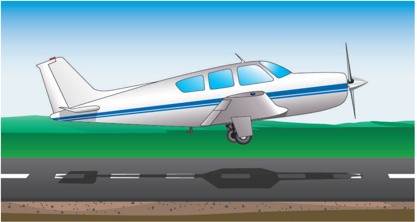
Figure 18-8. Landing with nose-wheel retracted.
