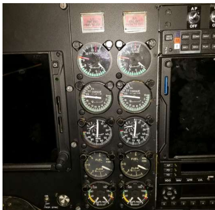
Figure 15-4. Powerplant instrumentation—fixed-shaft turboprop engine.
