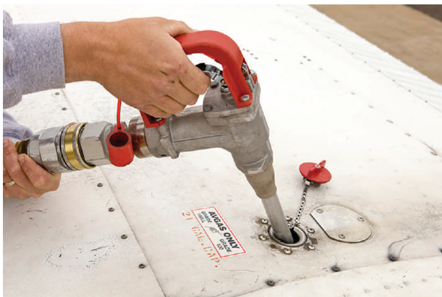
Figure 2-10. An AVGAS fuel filler nozzle is straight with a constant diameter.
