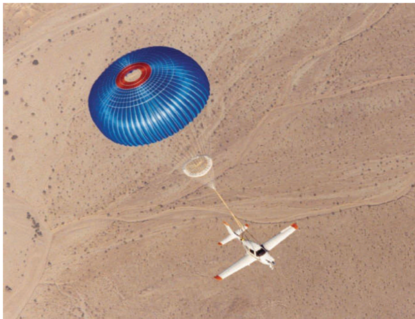
Figure 17-13. A ballistic recovery parachute is a popular safety feature available on some LSA.
